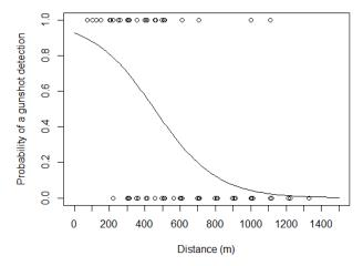
**Figure 6.** Fitted logistic regression of the probability of a gunshot being detected using the DTD 1.5.6 gunshot detection algorithm with threshold 0.4, plotted as a function of the acoustic sensor's (SWIFT rugged model) distance to the gunshot.
