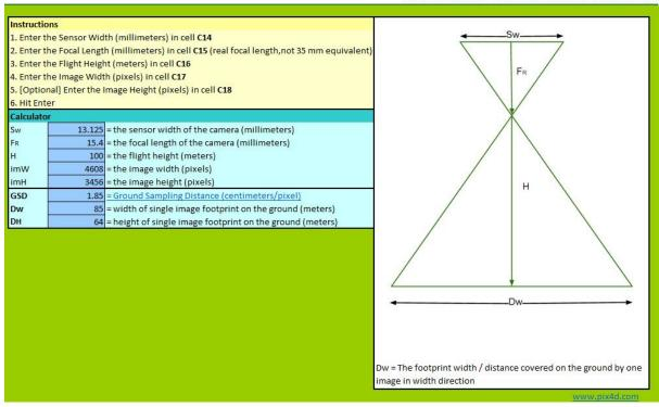
Pix4D ground sampling distance calculator. Source: Pix4D (https://support.pix4d.com/hc/en-us/articles/202560249-TOOLS-GSD-Calculator#gsc.tab=0)
