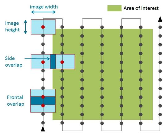
Schematic showing drone flight path over an area of interest. Image source: <a href="http://www.mining.com/web/how-a-sensor-gimbal-improves-efficiency-of-an-aerial-mapping-mission/">http://www.mining.com/web/how-a-sensor-gimbal-improves-efficiency-of-an-aerial-mapping-mission/</a>
